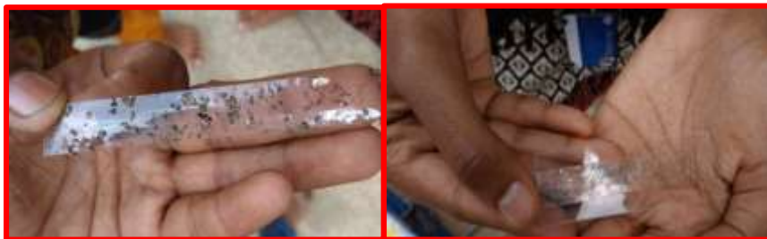
Fig 4: Sample collection using the Non-distractive adhesive tape method
