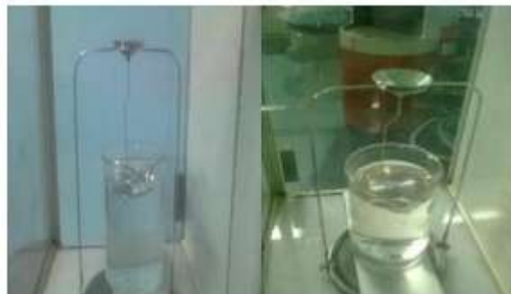
Fig. 1 Displacement method test for measuring the Density
