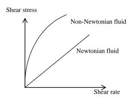
The viscosity of the fluid is defined as the ratio of the shear stress and shear rate. Thus the slope of the relation between shear-stress and shear-rate gives the viscosity  $(\eta)$ . If the plot
