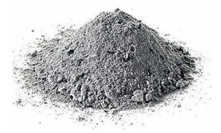
One of the key components of cow dung ash is silica. Silica is known to enhance soil properties such as compaction, strength, and resistance to moisture. Its presence in cow dung ash can contribute to improving the stability and load-bearing capacity of subgrade soils. Additionally, silica has a positive effect on reducing the plasticity and swelling potential of expansive soils, which are prone to volume changes with changes in moisture content.
