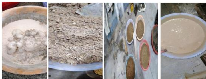
Figure 3: Sequential mixing of mortar material
