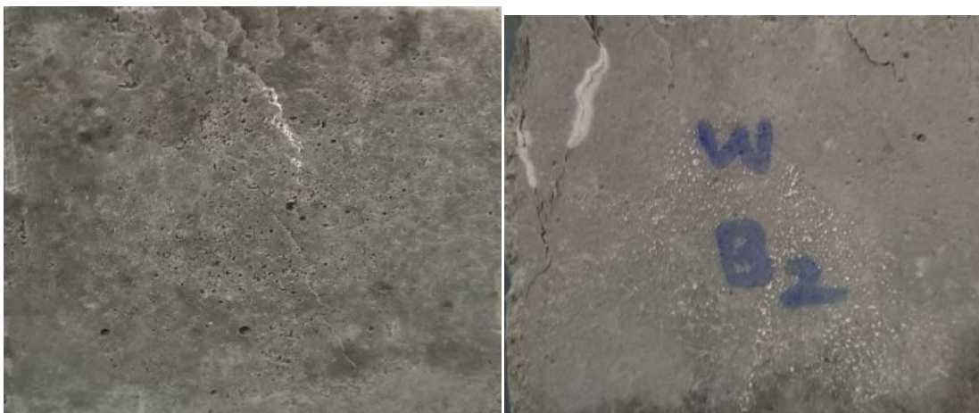
Fig. 2 Self-healing of concrete (formation of calcium carbonate)
