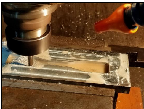
Fig 14. Visualization of the die manufacturing on the vertical milling machining
