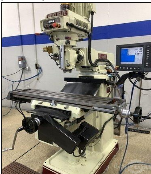
Fig 13. CNC vertical milling machine used for die and punch manufacturing
