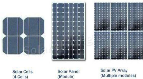
Fig 1. Arrangements of cell, module and array.
