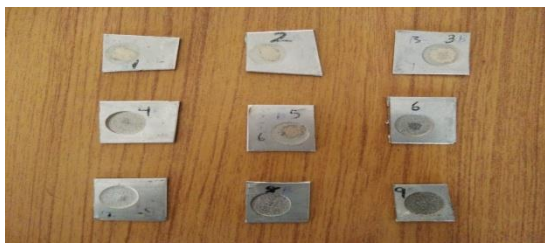
Fig.4 machining using brass as electrode
