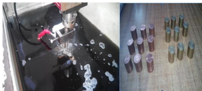
Fig. 3 Die Sinker EDM machining with tool and work piece (Model: ELEKTRA EMS 5535 MODEL)
