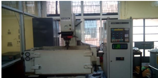
Fig. 2 Die Sinker EDM machine setup with tool and work piece (Model: ELEKTRA EMS 5535 MODEL)
