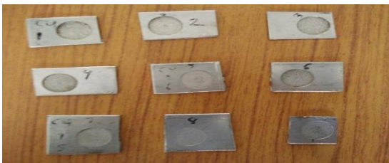
Fig. 5 machining using copper as electrode
