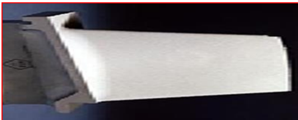
Fig.1 Gas Turbine blade with thermal barrier coating
