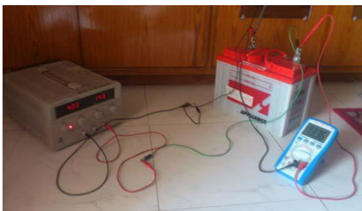
Figure 1.5.1 Setup of the battery for charging
