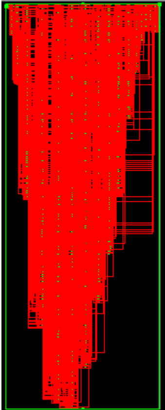
Fig.8: wallace multiplier with carry skip adder.
