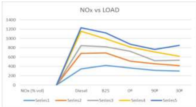
Figure6. LOADVS NO x AT 200 BAR & 23° BTDC
