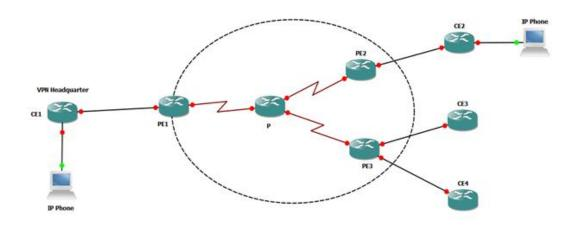
Fig 1 Architecture of MPLS-VPN
