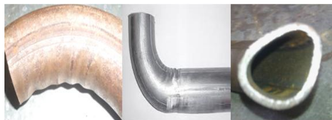
Fig.1 defects (wrinkling ,thining &oval) of the tube
