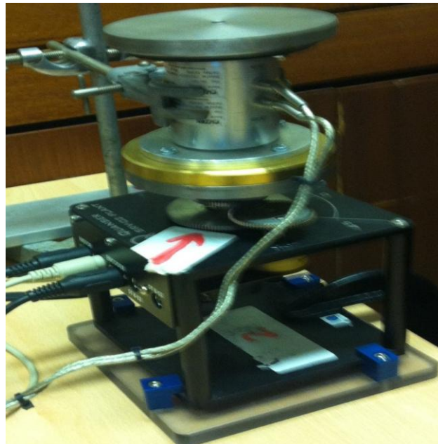
Fig. 1. The DC-servo motor friction test-bed
