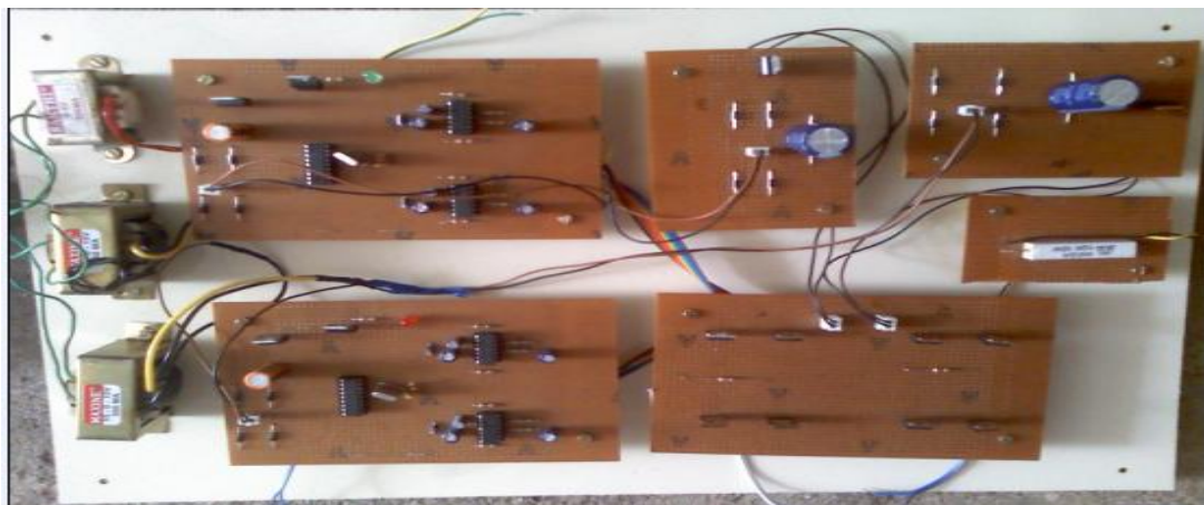
Figure 5. Hardware snap shot of seven level inverter
